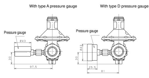
Note: Secure the space, at least, shown above before pressure adjustment. Be sure to detach the pressure gauge after pressure adjustment.
