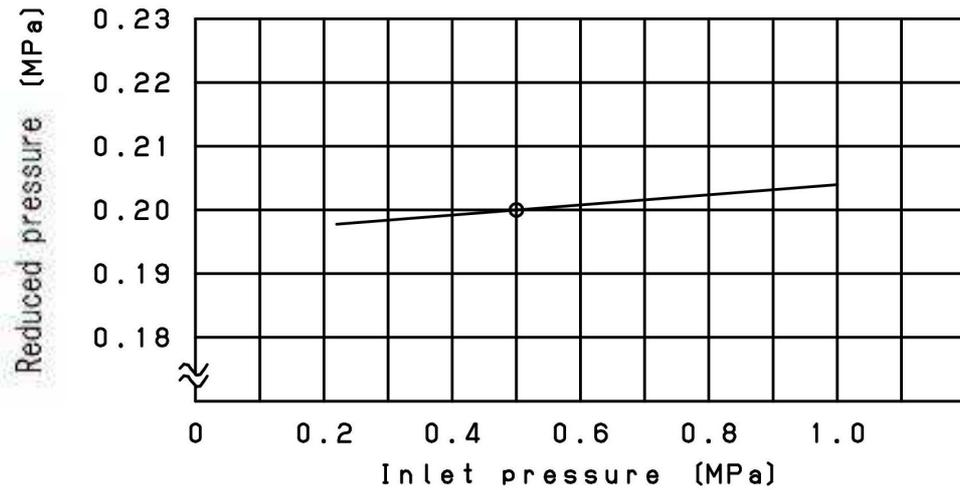
This chart shows variation in reduced pressure when the inlet pressure of 0.5 MPa is changed between 0.22 MPa and 1.0 MPa while the reduced pressure is set at 0.2 MPa.
