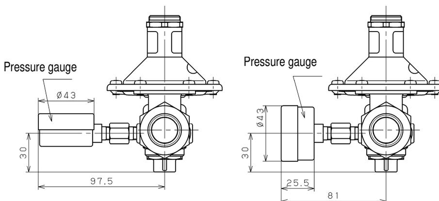
Note: Secure the space, at least, shown above before pressure adjustment. Be sure to detach the pressure gauge after pressure adjustment.
