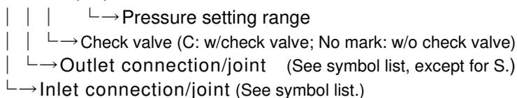
Note: "GD-46" with no symbols means parallel male threads (G1 x G1) for inlet and outlet.
