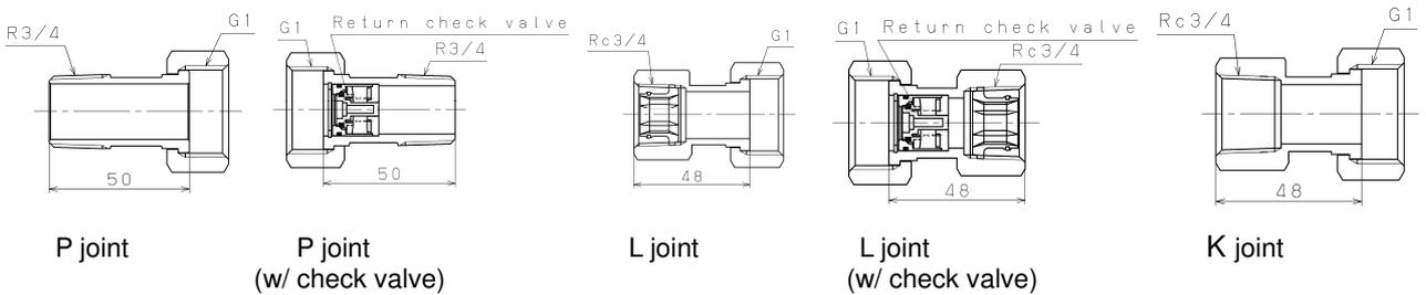
Note: Connections and joints depend on model.
