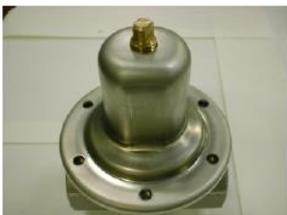
18) Insert spring washers and cross recessed pan head screws into the hole on the spring cover and Fully retighten the screws in an even, crisscross pattern.
