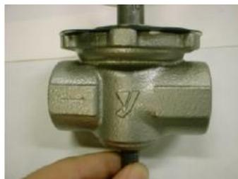
9) Remove valving element P, flat washer and hexagon nut. Go to step 10).
