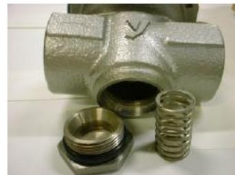
8) Applying, respectively but simultaneously, a socket wrench of nominal designation 10 to the U nut on the top of diaphragm and the hexagon nut on the valving element, remove the hexagon nut. Remove flat washer and then valving element P.
