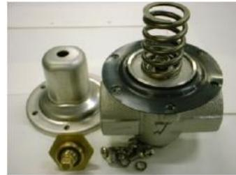
5) Verify that the diaphragm is damaged.
