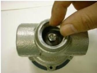
14) Apply socket wrench of nominal designation 10 to the U nut of the diaphragm and tighten the hexagon nut on valve element P by applying a torque of 6N-m (60 kgf·cm) to the torque wrench.
