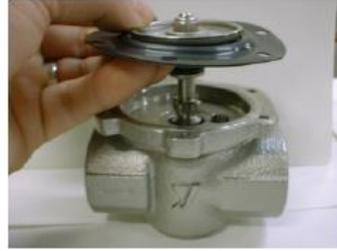
13) Place the valving element P, flat washer and hexagon nut onto the valve stem, and tighten by hand.
