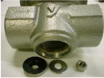
9'-1) Remove flat washer, diaphragm holding member and diaphragm in that order.
