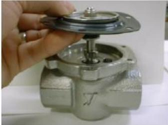
9'-2) Apply a suitable tool to the hexagon portion of the valve stem and remove the hexagon nut from the valving element P.
