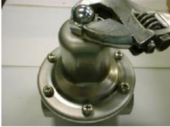
2) Turn dihedral adjusting screw counterclockwise to completely remove the spring load.
