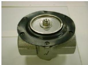
16) Place the adjusting screw on the adjusting spring.
