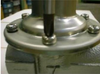
4) Remove spring cover, adjusting spring and adjusting screw.
