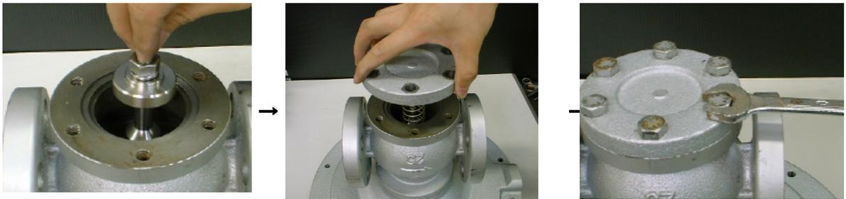
Action (19) : Attach O-ring ⑳, bottom diaphragm plate ㉑, diaphragm ㉒, top diaphragm plate ㉓ and washer ㉔. Position the holes of diaphragm ㉒. Tight locknut ㉕ manually.
