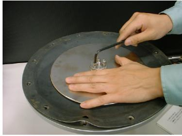
Action (21) : Place top diaphragm case ㉗. Align the holes of both components and secure the casing with 12 hexagon bolts ㉘. (Tightening torque: 18 N-m)
