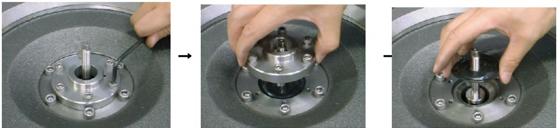
Action (31) : Replace balance diaphragm ⑦. Place top guide ⑧ and secure it with hexagon socket head cap bolt ⑨. **(Tightening torque: 5 N·m)**
