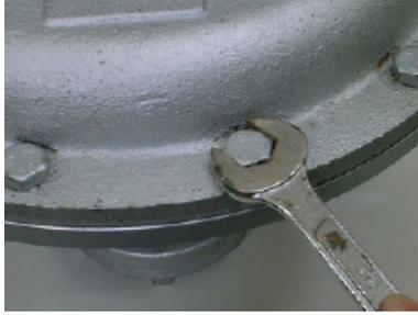
**Presumable cause III.19: Hexagon socket head cap bolt ㉔ and locknut ㉕ are loosened.**
