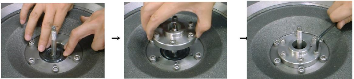
○Assembling the balance diaphragm
