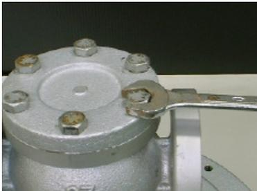
Action (39) : In the case the O-ring is damaged, unscrew hexagon head bolt ㉖ on the bottom cover.
