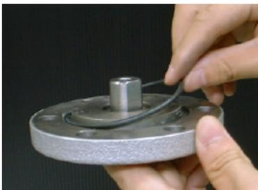
Action (40): Attach the bottom cover and secure it with hexagon head bolt ㉖.
