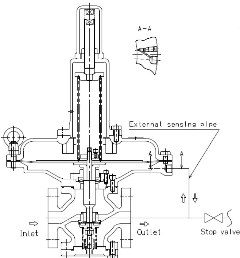
Gradually opening the outlet stop valve proportionally decreases the pressure applied on the diaphragm ②② until the load from the spring ②⑨ enables the disc ⑩ to open.
