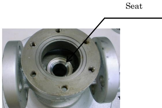
Action (15) : If the valve seat ② is damaged, consult us. If disc ⑩ is damaged, loosen hexagon nut ⑭ and remove spring washer ⑬ and valve ⑪. Remove the disc ⑩ from recess on the valve ⑪.
