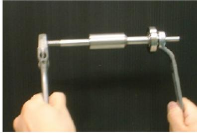
Action (18) : Attach spindle ⑫, disc ⑩, valve ⑪, spring washer ⑬, a set of hexagon nuts ⑭ and spring ⑮. Secure bottom cover ⑰ with 6 hexagon head bolts ⑱.
