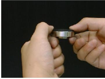
Action (17) : Attach disc ⑩, valve ⑪, spring washer ⑬ into spindle ⑫ and secure with hexagon nut ⑭.
