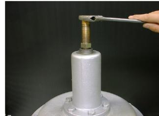
Action (9) : Unscrew 6 hexagon head bolts <sup>32</sup>. Remove spring chamber <sup>32</sup>, spring plate <sup>30</sup> and spring <sup>29</sup>.
