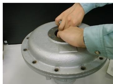
Action (11) : While securely holding top diaphragm plate ②③ with hand, unscrew 3 hexagon socket head cap bolts ②⑥.
