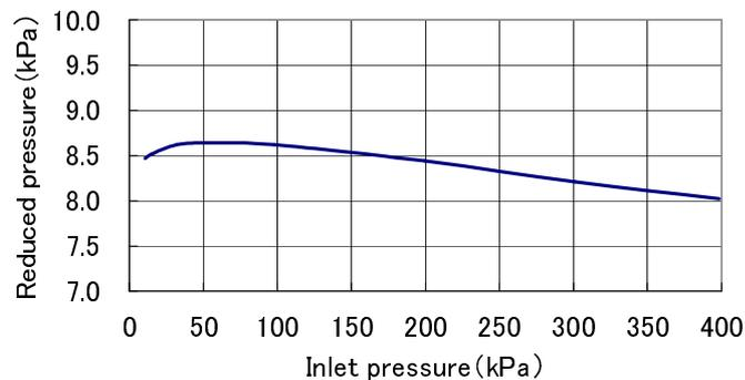
The chart shows changes in the reduced pressure when the inlet pressure is decreased from 400 kPa to 10 kPa with the reduced pressure set at 8.0 kPa.
