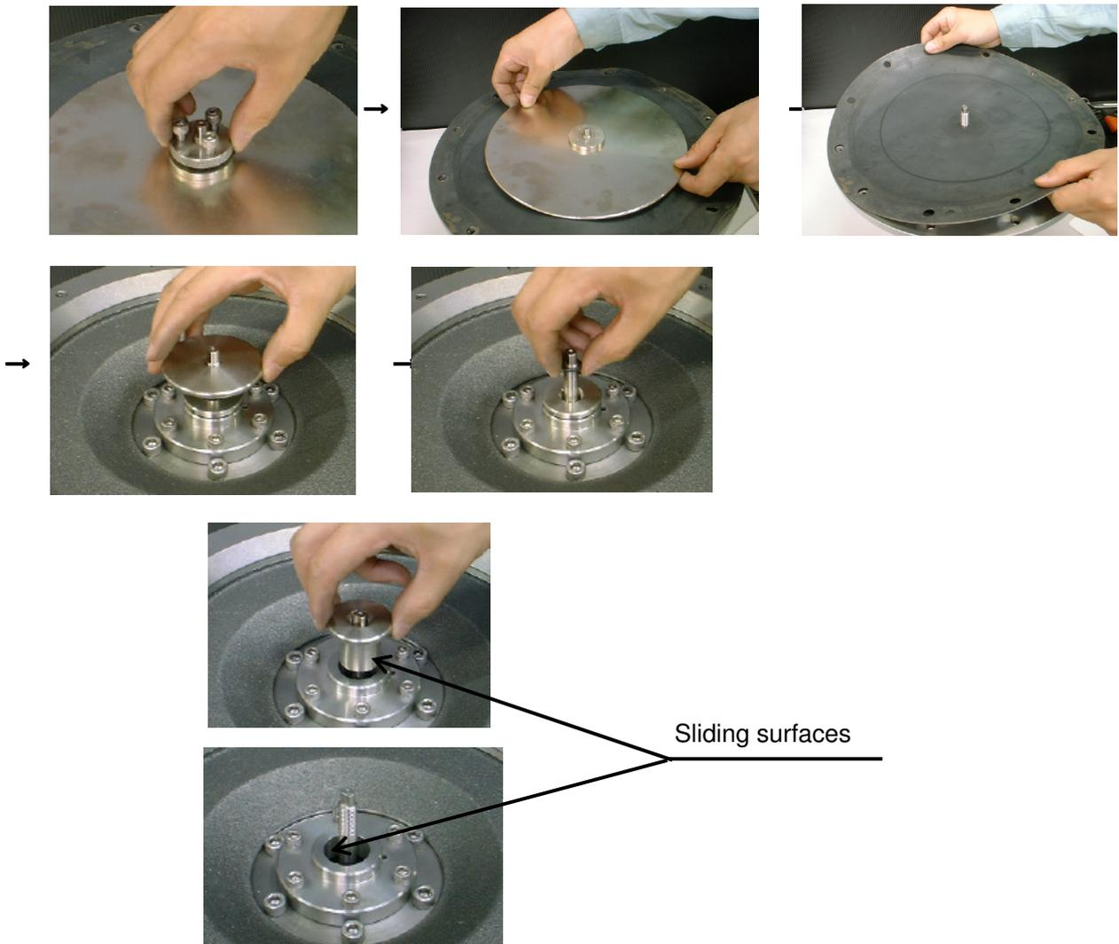
Action (13) : Remove 6 hexagon head bolts ⑬ from the lower cover. Remove spring ⑮, spindle ⑫, disc ⑩, valve ⑪, spring washer ⑬, and hexagonal nuts ⑭.
