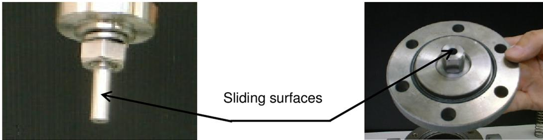
Action (14) : Check disc ⑩ and valve seat ② for pinched foreign materials and damage. Remove pinched materials, if any.
