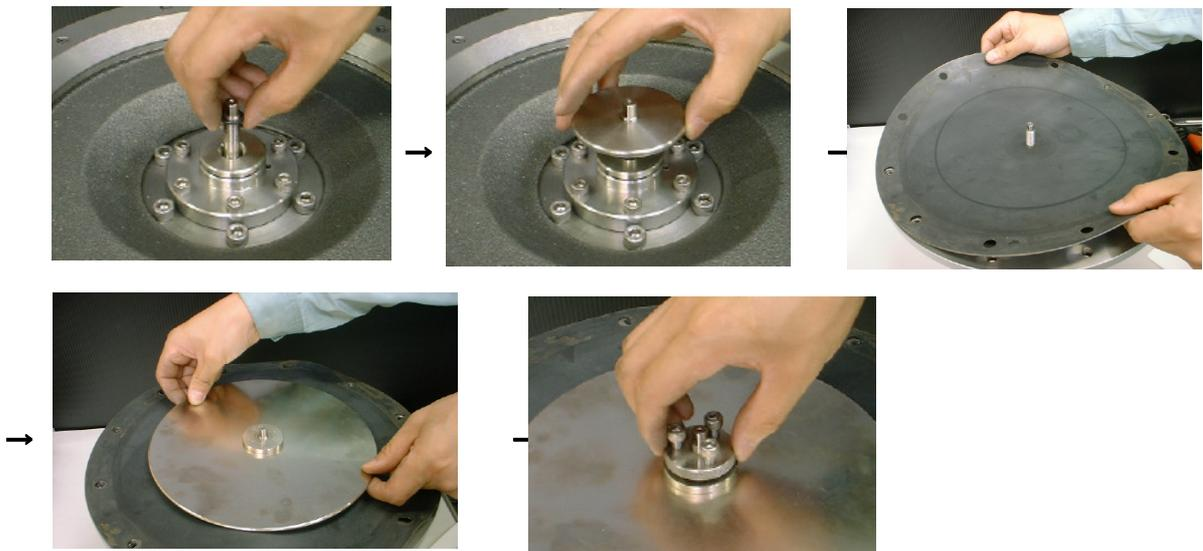
Action (20) : While securely holding top diaphragm plate ⑳ with hand, tighten 3 hexagon socket head cap bolts ㉔. (Tightening torque: 4 N-m)
