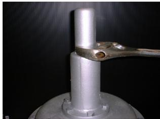
Action (8) : Loosen locknut <sup>33</sup>. Loosen bifacial adjusting screw <sup>34</sup> by turning it CCW to relieve the spring load.
