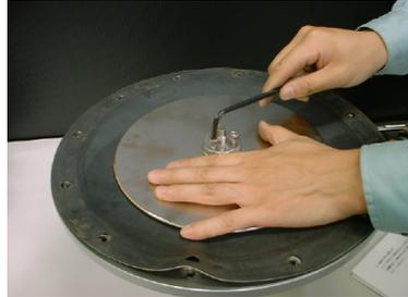
Action (12) : Loosen locknut ②⑤ and remove washer ②④, top diaphragm plate ②③, diaphragm ②②, bottom diaphragm plate ②① and O-ring ②⑦.
