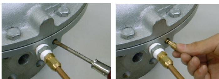
Action (5) : Clean the needle valve and hole of lower diaphragm casing.
