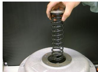
Action (10) : Loosen 12 hexagon head bolts <sup>40</sup> and remove top diaphragm case <sup>27</sup>.
