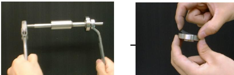
Action (16) : Place a new disc ⑩ in recess on the valve ⑪.
