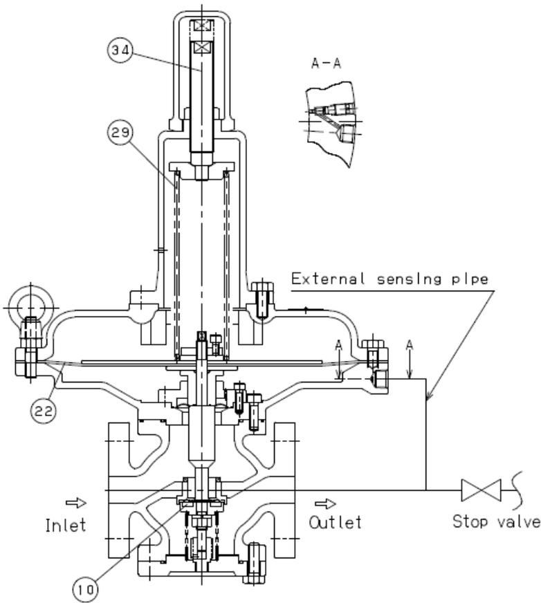
The adjusting screw ③④ compresses the adjusting spring ②⑨ to press down the diaphragm ②② that will open the directly connected disc ⑩.
