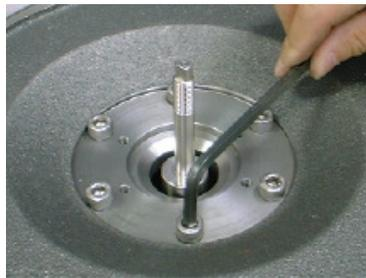
Action (45) : In the case O-ring is damaged, follow steps described in Actions (7) to (12). Unscrew hexagon head bolt ㉑. Remove the bottom diaphragm case and replace the O-ring.
