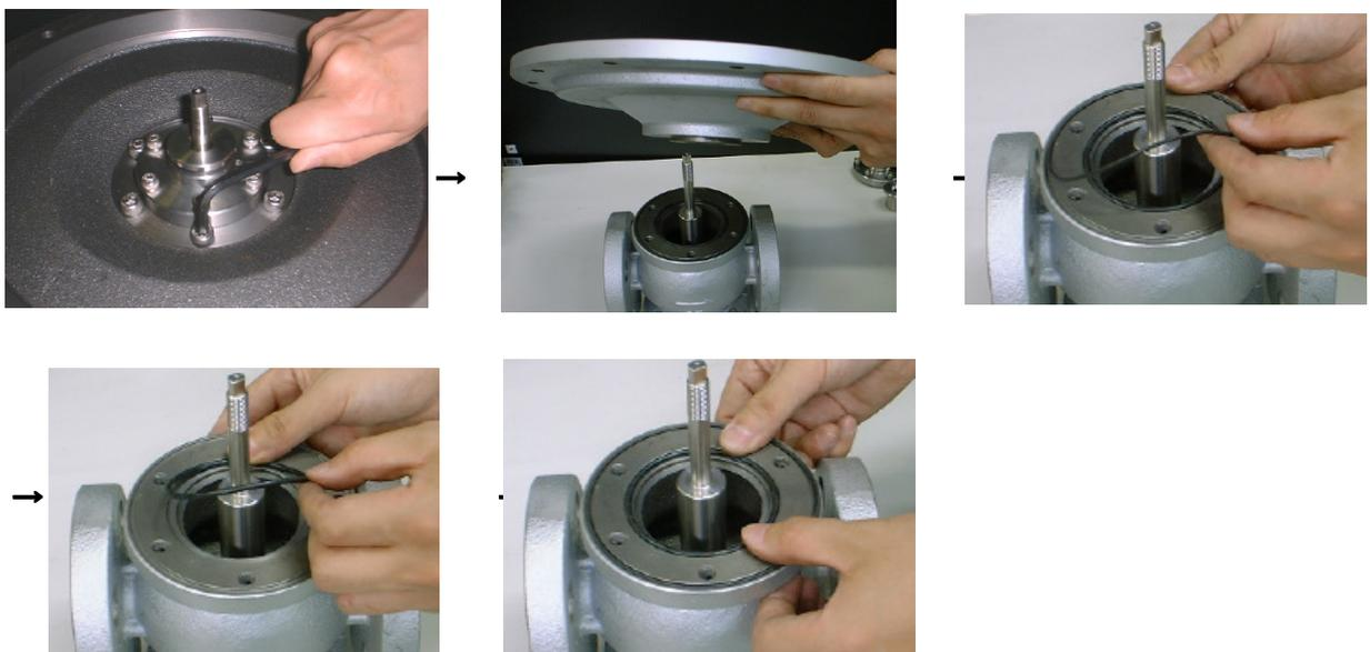
Action (46): Place the bottom diaphragm case and secure it with hexagon socket head cap bolt ⑥.
