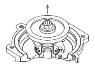
Nominal size 65A to 100A: Screw the bolt into the valve seat [3], and pull it up.
