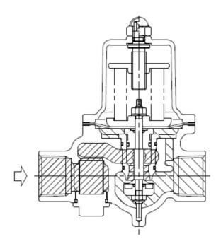
Gradually opening the sluice valve on the secondary side reduces the pressure applied to the diaphragm [9] and opens the disc [8]. The fluid flowing out to the secondary side acts on the diaphragm [9] as the secondary side pressure, balances with the load of the adjustment spring [15], adjusts the valve opening, and keeps the secondary side pressure constant.
