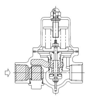
The adjusting screw [14] compresses the adjusting spring [15], pushes down on the diaphragm [9], and opens the disc [8] that is directly connected to it.
